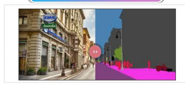
This is an example of a model in spatial sequencing, adaptable for radars, automated vehicles and other machines that need spatial recognition.
