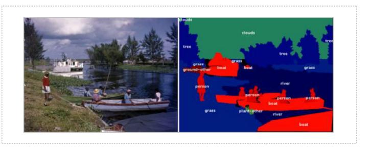
Image segmentation is the process of partitioning a digital image into multiple segments (sets of pixels, also known as image objects). The goal is to simplify and/or change the representation of an image into something that is more meaningful and easier to analyze. This is an example of model in spatial sequencing, adaptable for radars, automated vehicles and other machines that need spatial recognition.
